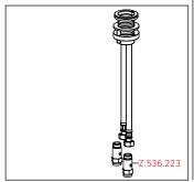
Flow rate normal spray 10 l/min (3 bar) Flow rate needle spray 9 l/min (3 bar) Acoustic group I
