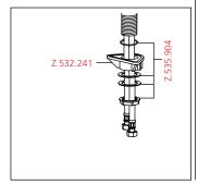
Flow rate normal spray 12 l/min (3 bar) Flow rate needle spray 11 l/min (3 bar) Acoustic group I
