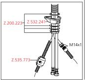
Flow rate normal spray 12 l/min (3 bar) Flow rate needle spray 13 l/min (3 bar) Acoustic group I
