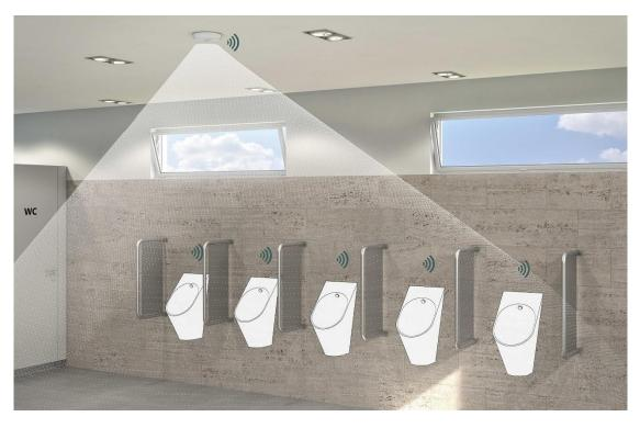
The ceiling-mounted Smart Urinal Sensor communicates wirelessly with the Smart Urinal Unit that is integrated behind the urinal and that consists of the locking water flow, solenoid valve and control unit for wireless communication in each case.
