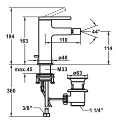
\* QuickInstallation - Fastening via threaded connection with locking
