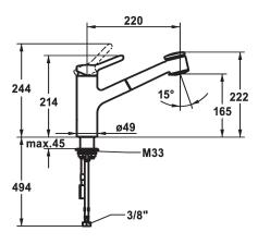
\* Hose guide, swivelling 130° \* EasyLock - a pull-out spray that easily slides back into place \* OptimalSpace - ample space for washing or working \* KWC cartridge M 35 H
