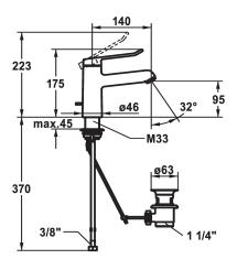
\* QuickInstallation - Fastening via threaded connection with locking
