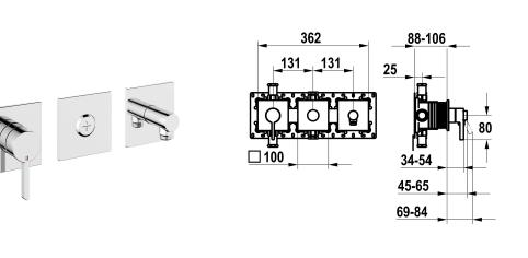
\* Scope of delivery: - Lever mixer unit - Diverter unit
