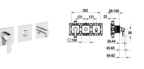
\* Scope of delivery: - Lever mixer unit - Diverter unit
